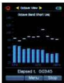
Real-time octave band screen with graphical display
