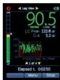
Leq screen with LAeq,t; Peak(C) & C-A values with the Leq value settled
