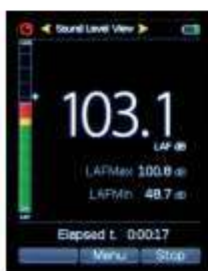
Sound Level Measurement Screen with Lmax & Lmin
