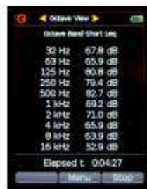
Real-time octave band screen with numerical display
