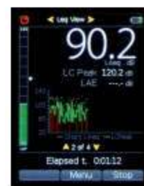
Leq screen with LAeq,t; Peak(C) and LAE
