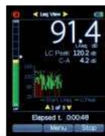
Leq screen with LAeq,t; Peak(C) & C-A values
